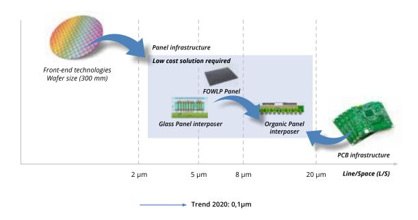
The heterogeneous integration domain in electronic components merges the conventional PCB with the wafer level technologies (source: Fraunhofer IZM).
