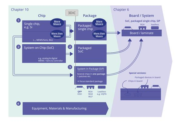
Close connection between electronics component development in this chapter with next level heterogeneous system integration in chapter 6
