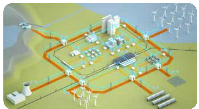
FIGURE 1 / Smart Energy landscape – from centralized to distributed (PV, wind, biogas, ...) generation and conversion, consisting of High/Medium Voltage grid (orange), Low Voltage grid (yellow) including Communication Network (aquamarine) linking producers and consumers down to regional and community level (source ECSEL MASP 2016 9 )
